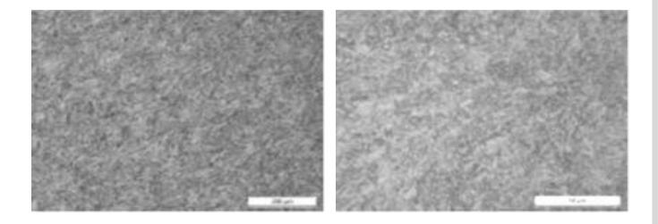
Heat-treated microstructure at the core of the sample. Uniform, fine-tempered martensitic microstructure is observed.
